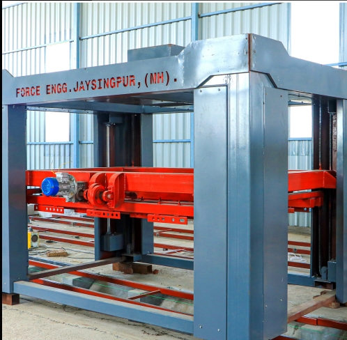
WIRE CUTTING MACHINE
